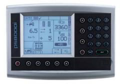
The **RDS Artemis** is a variable rate control and monitoring system for seed drills that removes the need for a mechanically driven land wheel by operating the metering unit with an electric motor maintaining its speed proportional to forward speed.
