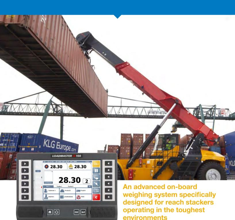
The RDS **LOADMASTER CL100** is a CAN based system setting a benchmark for the industry, combining cutting edge sensor technology and signal processing techniques providing precise and consistent weight information.
